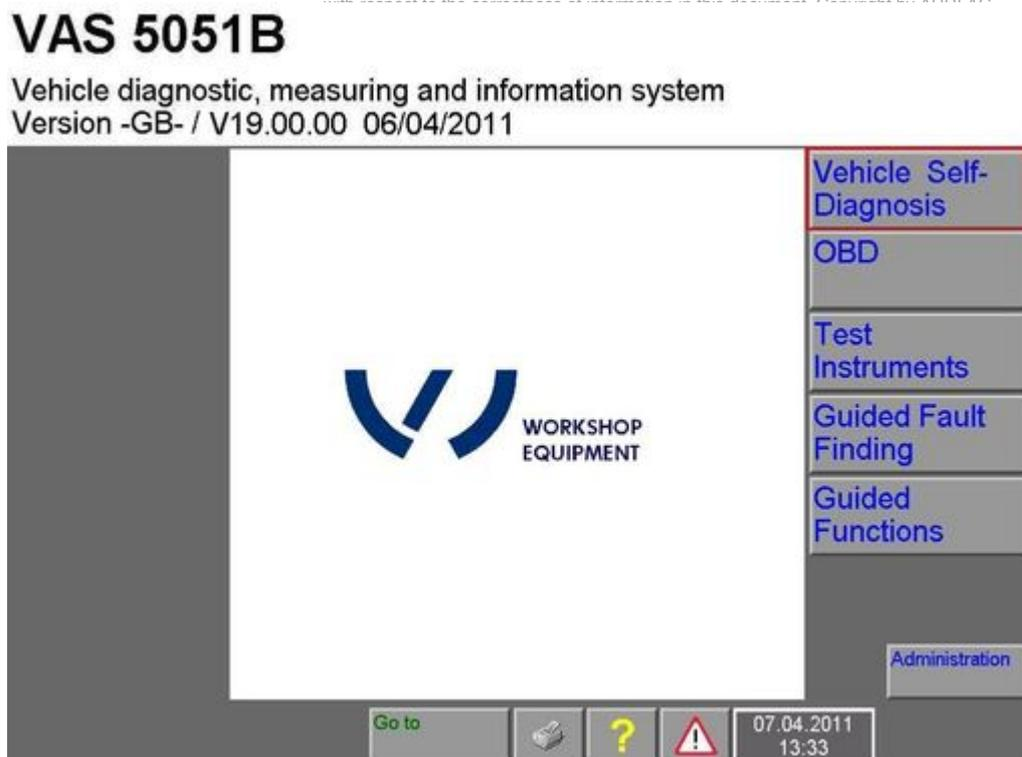
Figure 1-1 Start mask, activating “*Vehicle self-diagnosis*”
