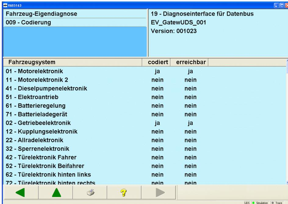
Figure 3-80 Coding installation list
