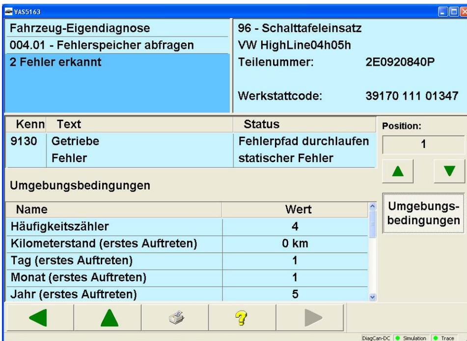
Figure 3-24 Checking DTC memory, displaying environment conditions
