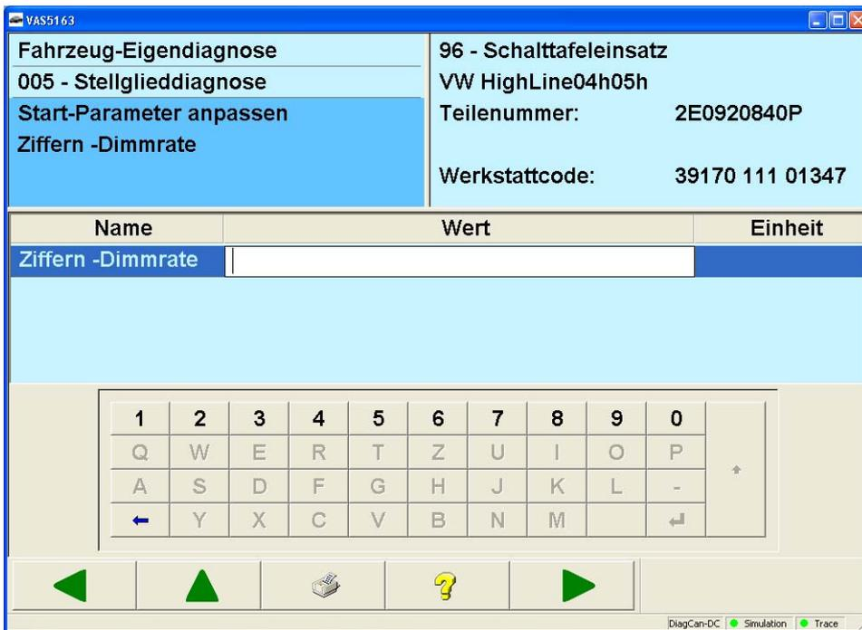
Figure 3-35 Adapt start parameters in the Crafter final control diagnosis
