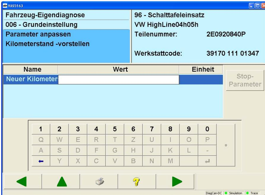
Figure 3-61 Carry out the parameterisation of the basic setting
