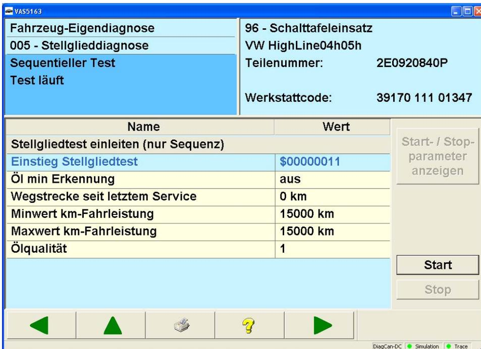
Figure 3-38 Sequential test, test is running (Crafter final control diagnosis)
