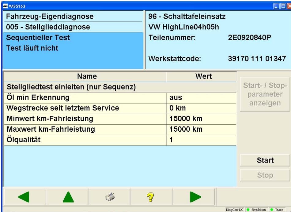
Figure 3-37 Sequential test, test does not run (Crafter final control diagnosis)
