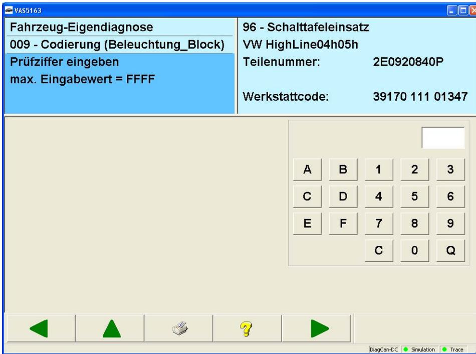
Figure 3-74 Enter test character for the Crafter coding
