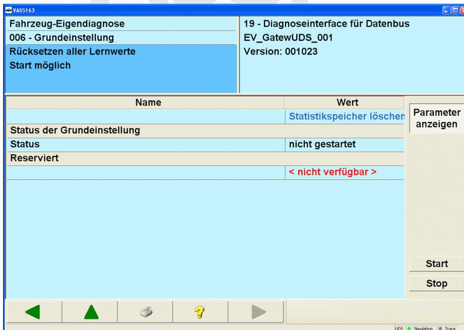
Figure 3-57 UDS basic setting, does not run
