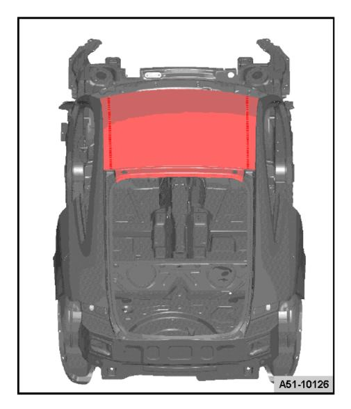
Remove the remainder on the roof frame using the single hand angle grinder -VAS 5167- .
