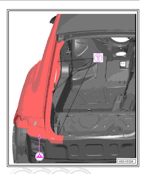
Crimp the wheel housing with the fold crimping tool -V.A.G 1585- .
