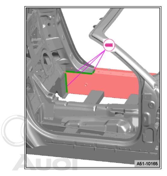
Weld the inner lower still panel with a SG continuous seam or accept any liability using the gas-shielded welder 250A -VAS 6388- document. Copyright by AUDI AG.
