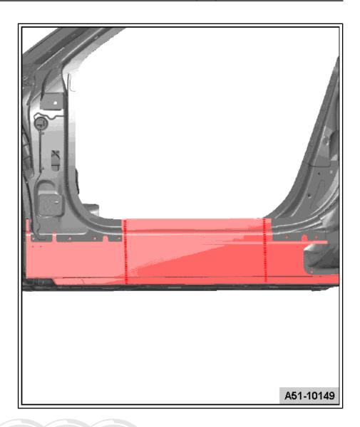
Make the separating cuts using the body repair saw -V.A.G 1523A- as shown.
