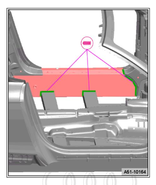
Weld the inner lower sill panel with a SG continuous seam using the gas-shielded welder 250A -VAS 6388- .
