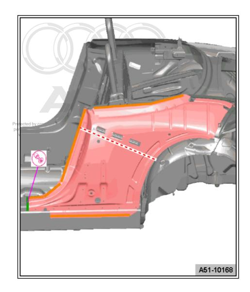
Remove the remainder using the single hand angle grinder - VAS 5167- .
