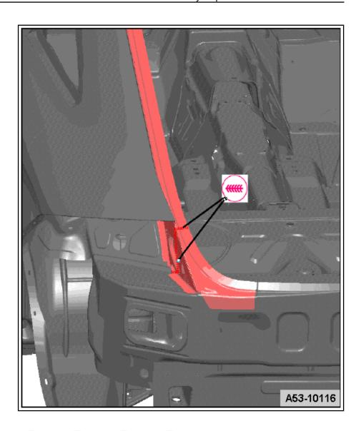
Weld the rain water drain channel reinforcement with a SG continuous seam using the gas-shielded welder 250A -VAS 6388- .
