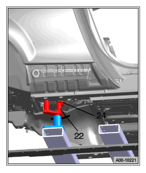
22 -24 - Rear suspension strut mount Overview of rear alignment bracket positions
