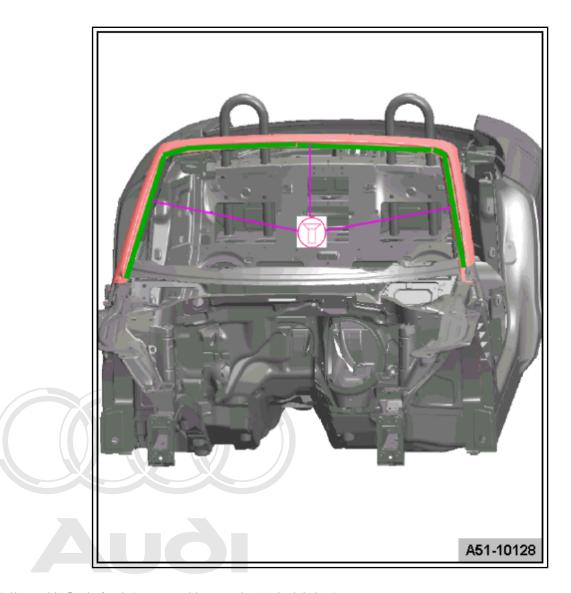
Rivet the root frame with a rechargeable riveter of AS 5279/2 - or the rechargeable riveter -VAS 5279B- with D15 and D16 punch .
