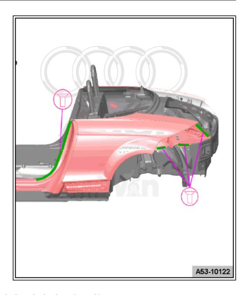
Rivet in the rain water drain channel using the rechargeable riveter -VAS 5279A- .
