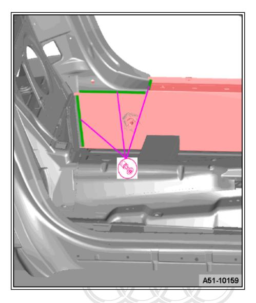
Remove the sill panel strip inner original joint using the straight sander -VAS 5170- .
