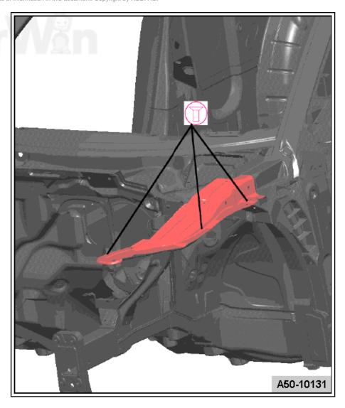
Attach the connection to the A-pillar using an M5 x 18 flange bolt.
